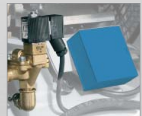
PPS control unit (PERMANENT-POWER-SYSTEM)
